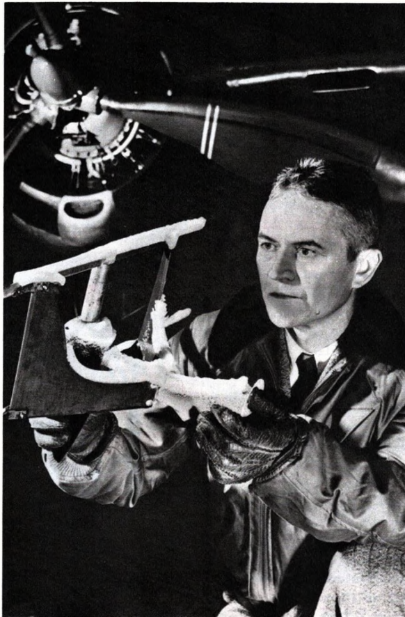
Mr. Rodert examines ice collected on plane's radio antenna after an experimental flight
